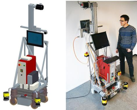
**Figure 4:** Mobile scanning system
